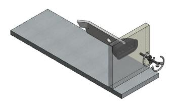
Drill the formwork and push the TBV or TDV into the designated hole, screw the recess former RBF in with the anchor mounted. Pull to formwork and tighten against the formwork using the second nut.
